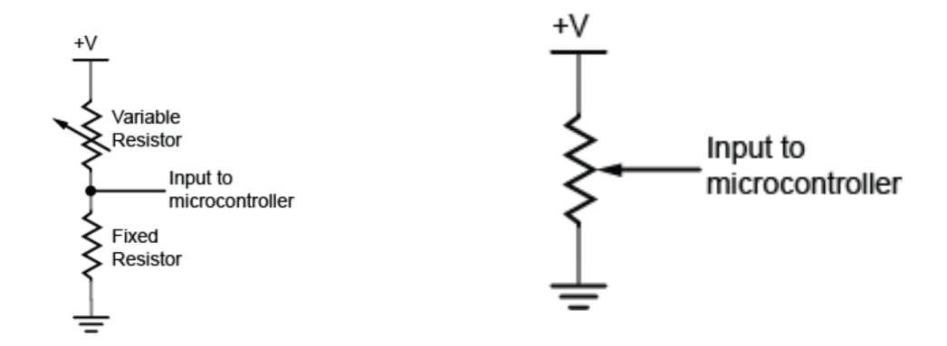
An input that can read a variable voltage, typically from 0 volts to the maximum voltage that powers the microcontroller itself.
